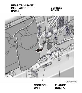
19. Remove the tape to free the vehicle 12-pin connector and plug it to the control unit.
