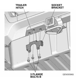
Install the socket harness to the socket bracket with the two flange bolts B.
