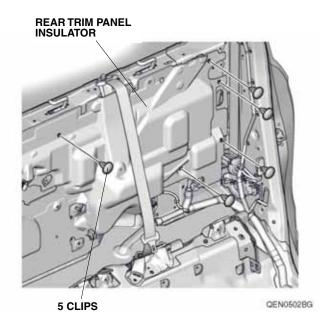
18. Peel the rear trim panel insulator. Secure the control unit to the vehicle panel with one flange bolt A.
