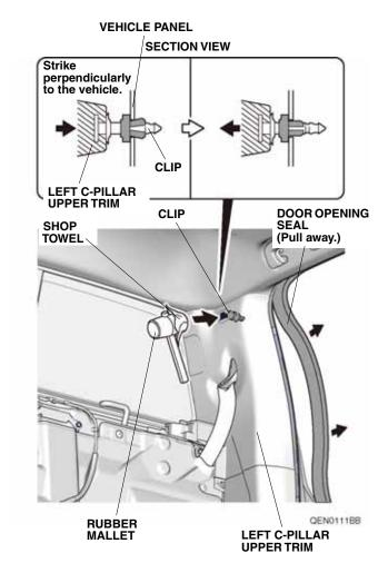
13. Using a rubber mallet wrapped with a shop towel, lightly tap the area marked SIDE CURTAIN AIRBAG on the left C-pillar upper trim to push in the clip. NOTE: Make sure to strike the area perpendicular to the vehicle.
