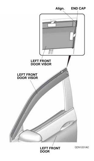
10. While applying light pressure against the left front door visor, carefully remove the adhesive backings in the order shown. Make sure to push up on the brackets while removing the adhesive backings. NOTE: While removing the long top adhesive backing, make sure the left front door visor is positioned so the top edge of the vehicle chrome is hidden by the left front door visor.
