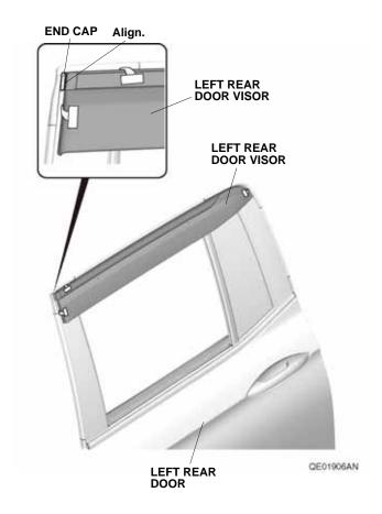
20. While applying light pressure against the left rear door visor, carefully remove the adhesive backings as shown. Make sure to push up on the brackets while removing the adhesive backings. NOTE: While removing the long top adhesive backing, make sure the left rear door visor is positioned so the top edge of vehicle chrome is hidden by the left rear door visor.
