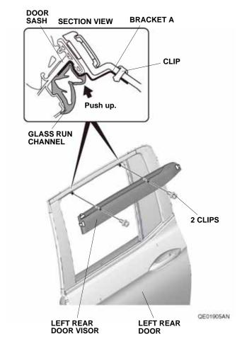
18. Secure the left rear door visor to two brackets A with two clips. Make sure to push up on the two brackets A while installing the two clips.
