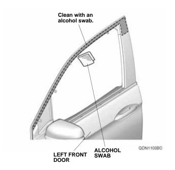
Attach a piece of masking tape to the end of the adhesive backings as shown. Peel back the adhesive backings partway and temporarily attach them to the front surface of the left front door visor.
