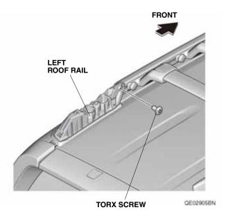
7. Install the roof rail covers. Make sure they are securely snapped in place.
