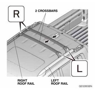
Line up the marks on the crossbars with the marks on the roof rails as shown. Tighten the eight thumbwheel screws to secure the crossbars to the roof rails.
