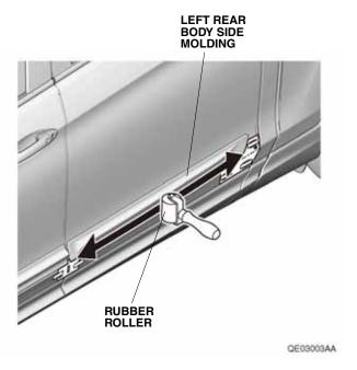
14. Remove the templates. Turn the templates over and repeat steps 1 through 13 to install the right body side moldings.
