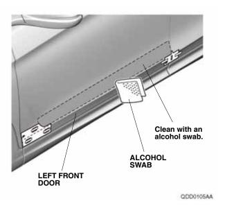
5. Peel back the adhesive backings and tape them to the front surface of the left front body side molding. Remove the remaining adhesive backings.
