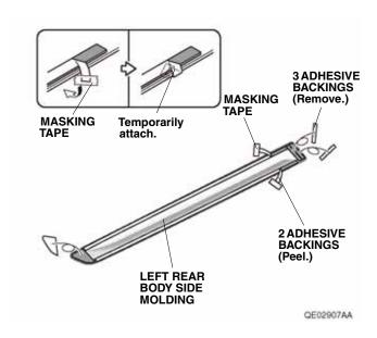
11. Line up the left rear body side molding with the middle and rear templates and attach it to the left rear door as shown.
