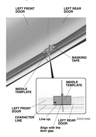
3. Fold the tab, line up the rear template with the character lines and attach it to the left rear door with masking tape as shown.
