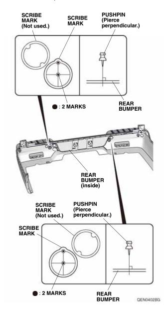
67. While wearing eye protection, drill the eight pierced marks with a 3 mm drill bit from the painted side of the rear bumper.
