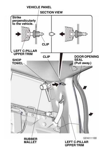
Using a rubber mallet wrapped with a shop towel, lightly tap the area marked "SIDE CURTAIN AIRBAG" on the left C-pillar upper trim to push in the clip.
