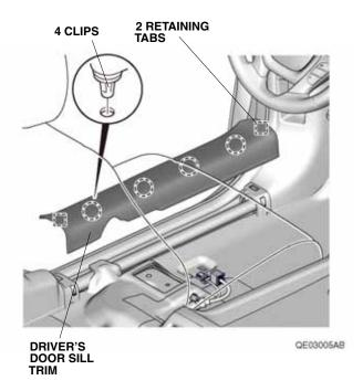
5. Pull away the door opening seal and remove the driver's kick panel.
