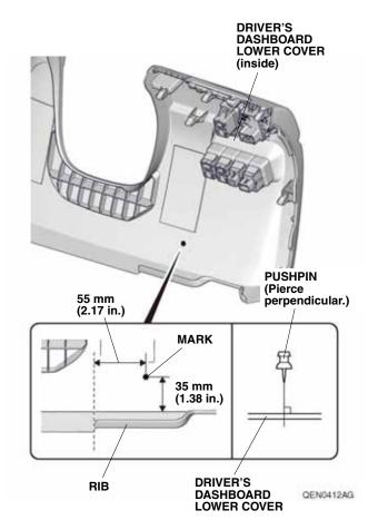
81. While wearing eye protection, drill the pierced mark on the driver's lower cover with a 3 mm drill bit. NOTE: Make sure to drill perpendicular to the driver's dashboard lower cover.
