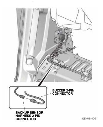
53. Bundle up the excess buzzer harness and secure the buzzer harness and backup sensor harness to the vehicle panel with one wire tie with clip A and one wire tie with clip B.
