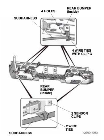
78. Secure the subharness to the two sensor clips with two wire ties.
