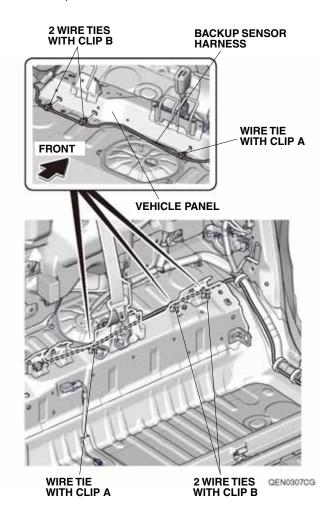
44. Secure the backup sensor harness to the vehicle panel with three wire ties with clip B.
