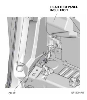
46. Using a utility knife, cut off the rear trim panel insulator as shown.
