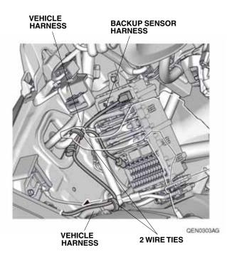
39. Secure the backup sensor harness to the vehicle harness with three wire ties.
