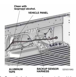
Secure the backup sensor harness to the vehicle panel with one aluminum tape as shown. 59. Secure the backup sensor harness to the vehicle panel and vehicle harness with one wire tie with clip A and three wire ties.
