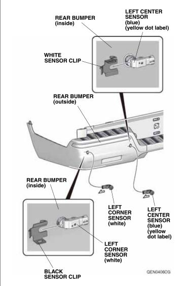
71. Secure the left corner sensor (white) and left center sensor (blue) with white sensor clip and black sensor clip as shown.
