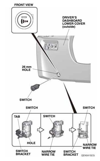
84. Align the tab on the switch bracket with the hole on the switch and secure the switch bracket to the switch with one narrow wire tie.
