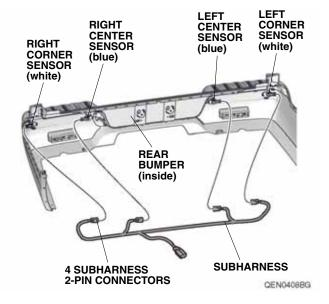
75. Secure the subharness to the four tabs on the rear bumper.
