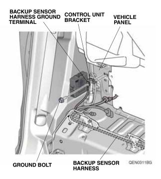
Plug the backup sensor harness 14-pin connector into the control unit.
