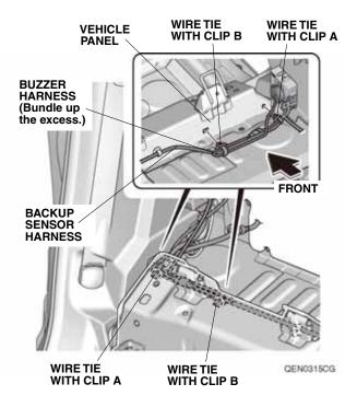
54. Remove the vehicle grommet. Route the backup sensor harness through the vehicle grommet hole. Install the floor carpet.
