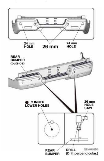
Insert the left corner sensor (white) and left center sensor (blue) into the rear bumper.
