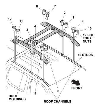
10. Install the roof rack to the roof channel with 12 T-30 Torx nuts in the order shown. Torque the Torx nuts to 10 N·m (7.4 lbf·ft).
