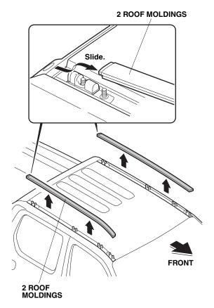
Using long nose pliers, remove six clips from the roof channels. Discard the clips.
