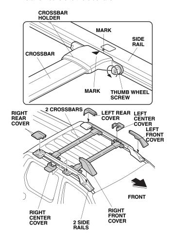
Loosen four thumb wheel screws on the crossbar holders. Align the marks on the crossbar holders with the marks on the side rails. Securely tighten the thumb wheel screws.
