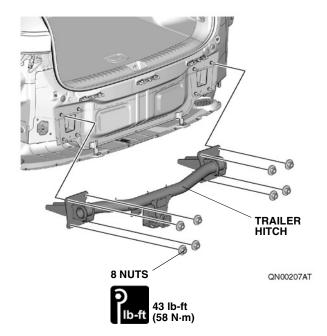
Install the reinforcement plates to the frame under side and secure the trailer hitch with the supplied M12 x 1.75 bolts.
