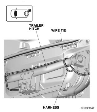
28. Remove the self-tapping screws and vehicle harness (with hands-free access).
