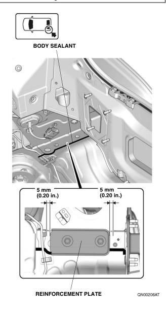
16. With the aid of an assistant, insert the trailer hitch into the body rails. Secure the trailer hitch with the retained impact bar nuts. Tighten the nuts using a cross pattern from left side to right side to ensure an even load distribution.
