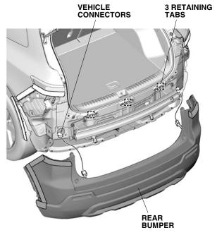
12. Remove the self-tapping screws and vehicle harness (with hands-free access).
