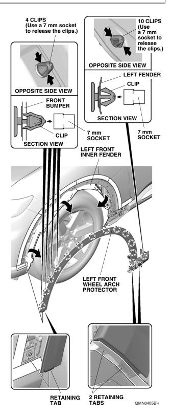
5. Remove the clips and spring nut.
