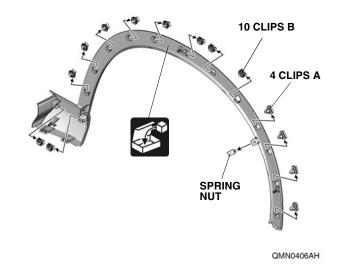
6. Install the clips and spring nut.
