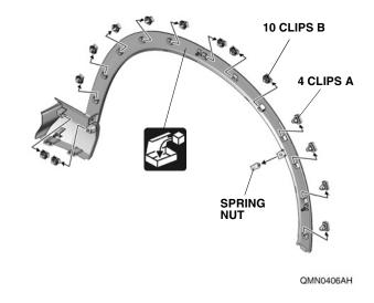
6. Install the clips and spring nut.
