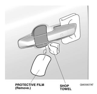
9. Wipe off the 3M protective tape application solution.
