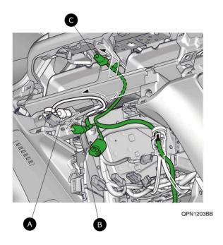
A VEHICLE 4-PIN CONNECTOR (with masking tape)
