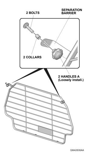
9. Install the separation barrier.
