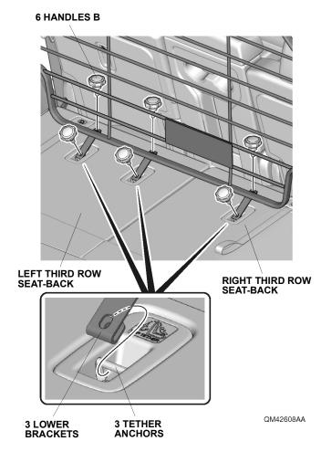
12. Secure the separation barrier.
