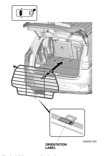
10. Install the separation barrier.
