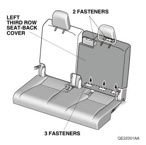
8. Secure the left third row seat-back cover with the fastener. Secure the strap to the left third row seat-back cover with the fastener.
