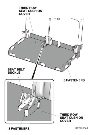
12. Insert the third row seat cushion cover between the third row seat-back and third row seat cushion. Make sure to insert the third row seat cushion cover under the anchors. Secure the fasteners to the third row seat cushion.
