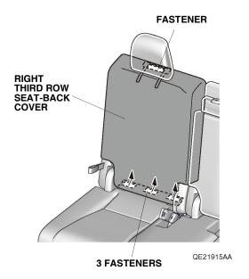
Secure the right third row seat-back cover with the fastener. Secure the strap to the right third row seatback cover with the fastener.
