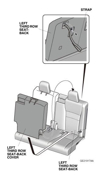
Secure the left third row seat-back cover with the fasteners.
