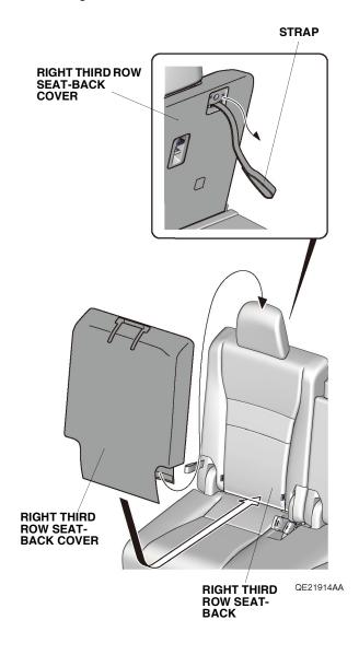
Secure the right third row seat-back cover with the fasteners.
