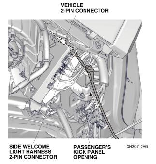
47. Secure the side welcome light harness to the vehicle harness with two wire ties.
