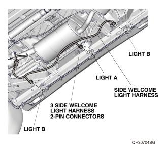
38. Secure the side welcome light harness to the one trim A, two trim B, and right side sill panel with seven wire ties as shown.
