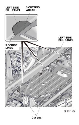
11. Remove the undercoating as shown. Apply touch-up paint where you removed the undercoating and allow it to dry thoroughly.
