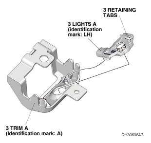
15. Install the three retainers to each trim A with three self-tapping screws as shown.
