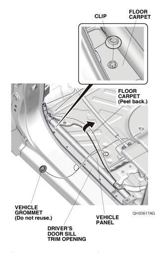
24. Remove the vehicle grommet from the vehicle panel.
