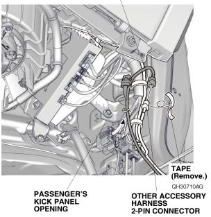
50. Bundle up the excess side welcome light harness, and secure it and 2-pin connectors to the vehicle harness with two wire ties as shown.
