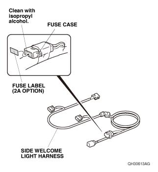
37. Plug the three side welcome light harness 2-pin connectors into the one light A and two lights B.
