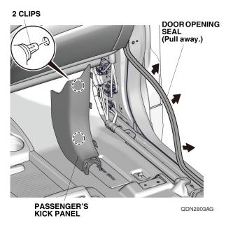
6. Pull away the door opening seal, and remove the driver's dashboard side lid.
