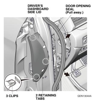
7. Remove the driver's dashboard lower cover, and unplug the vehicle connectors, and release the vehicle sensor.
