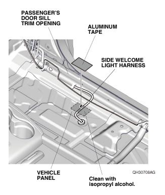
44. Secure the side welcome light harness to the vehicle panel with one aluminum tape as shown.
