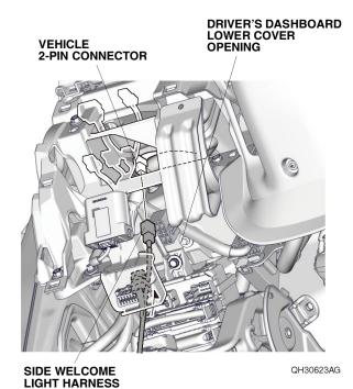
31. Secure the side welcome light harness to the vehicle harness with two wire ties.
