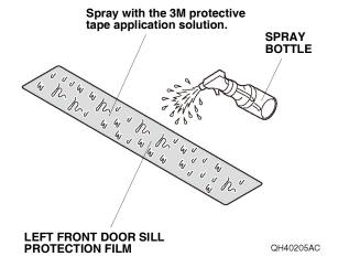
6. Line up the left front door sill protection film with the curve end and masking tape as shown. Then, attach it to the vehicle panel.
