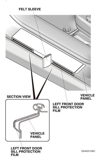
Using a shop towel, wipe off the 3M protective tape application solution. Allow the left front door sill protection film to dry thoroughly. Remove the masking tape.
