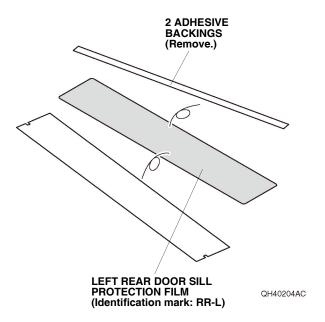
16. Spray the left rear door sill protection film with the 3M protective tape application solution.
