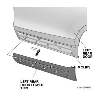
Remove the nine clips from the left rear door as shown.
