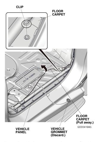
31. Locate the vehicle grommet, and remove it from the vehicle panel.
