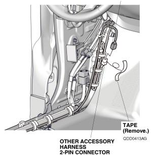
26. Bundle up the excess left running board harness, and secure it to the vehicle harness with two wire ties. Go to step 30.
