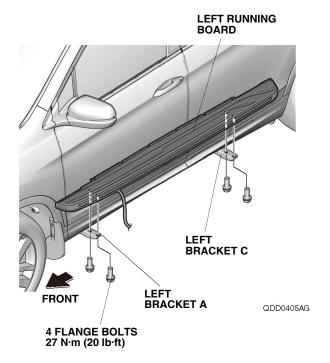
13. Tighten the four flange bolts loosely installed in step 11. Torque the flange bolts to 27 N·m (20 lb·ft).
