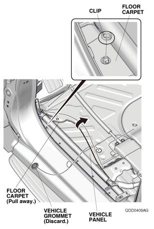
19. Locate the vehicle grommet, and remove it from the vehicle panel.
