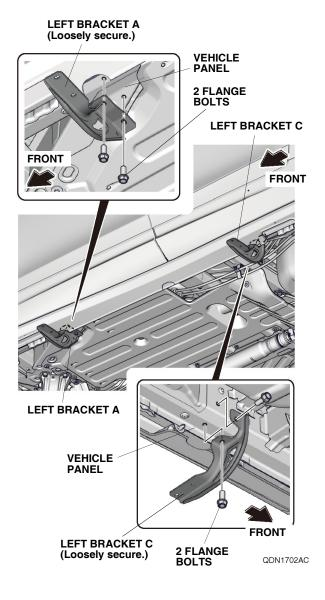
Secure the left running board to the left bracket A and left bracket C with four flange bolts. Torque the flange bolts to 27 N·m (20 lb·ft).
