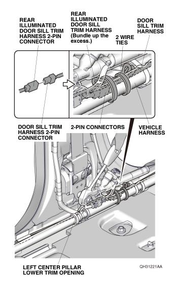
50. Bundle up the excess rear illuminated door sill trim harness, and secure it and the 2-pin connectors to the vehicle harness with two wire ties as shown.
