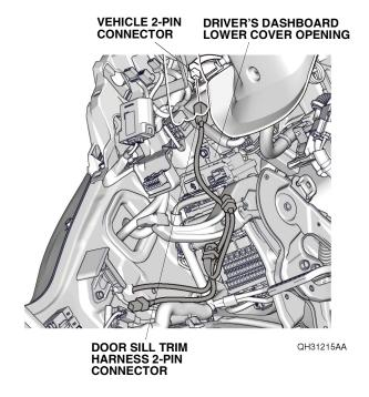
43. Secure the door sill trim harness to the vehicle harness with two wire ties.
