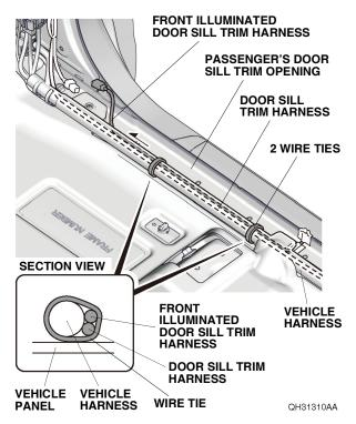
72. Plug the door sill trim harness 2-pin connector into the front illuminated door sill trim harness 2-pin connector, and secure the 2-pin connectors and door sill trim harness to the vehicle harness with one wire tie.
