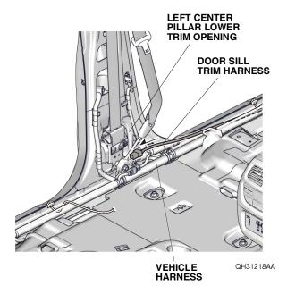
46. Using isopropyl alcohol on a shop towel, thoroughly clean the vehicle panel where the aluminum tape will attach.
