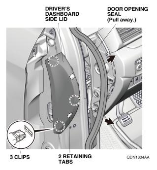
6. Remove the driver's dashboard lower cover, and unplug the vehicle connectors, and release the vehicle sensor.
