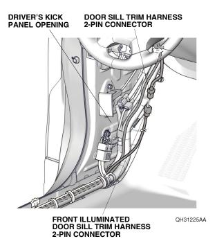
56. Bundle up the excess front illuminated door sill trim harness, and secure it and the 2-pin connectors to the vehicle harness with three wire ties as shown.
