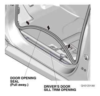
20. Using an alcohol wipe, thoroughly clean the vehicle panel where the front illuminated door sill trim will attach.
