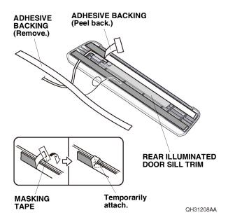
30. Line up the rear illuminated door sill trim with the masking tape. Attach the rear illuminated door sill trim to the vehicle panel.
