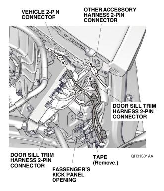
58. Remove the tape to free the door sill trim harness 2-pin connector, and plug it into the other accessory harness 2-pin connector.
