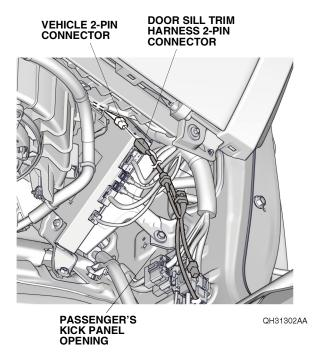
Secure the door sill trim harness to the vehicle harness with three wire ties.
