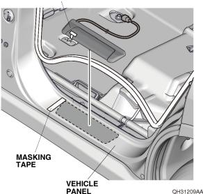
31. While applying light pressure against the rear illuminated door sill trim, carefully remove the taped adhesive backing.
