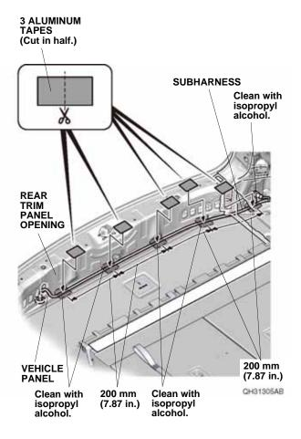
42. Using scissors, cut three aluminum tapes in half, and secure the subharness to the vehicle panel with five pieces of aluminum tape as shown.
