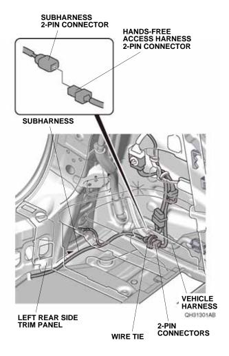
Secure the 2-pin connectors to the vehicle harness with one wire tie.
