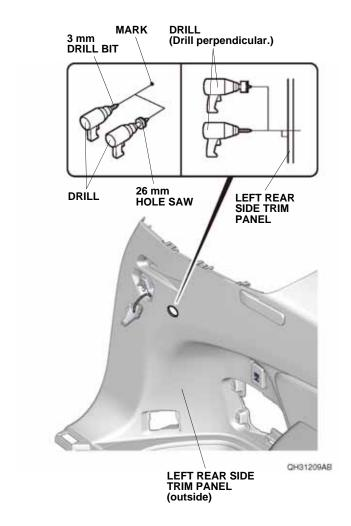
21. Install the switch into the 26 mm hole. NOTE: Make sure to install the switch in the correct orientation.
