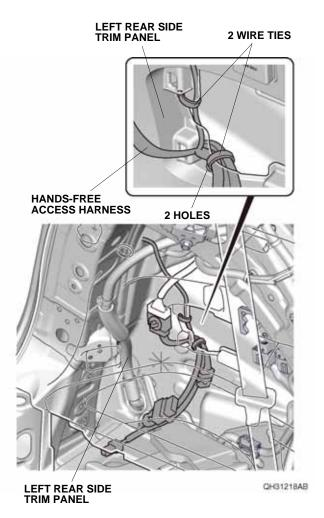
34. Route the subharness as shown. Plug the handsfree access harness 2-pin connector into the subharness 2-pin connector.
