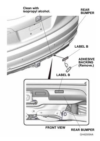
62. Remove the adhesive backing from the label B, and attach the label B to the rear bumper as shown. NOTE: Make sure the customer is aware that label B can be removed after reading.
