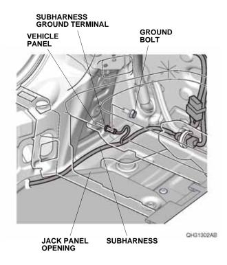
37. Remove the vehicle grommet. Route the subharness through the vehicle panel hole as shown.
