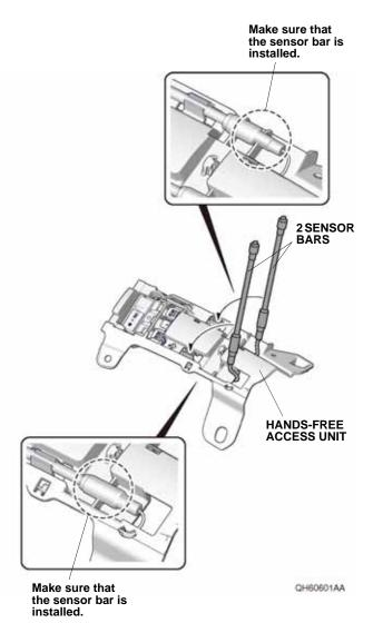
48. Make sure the sensor bar wires are secured as shown.
