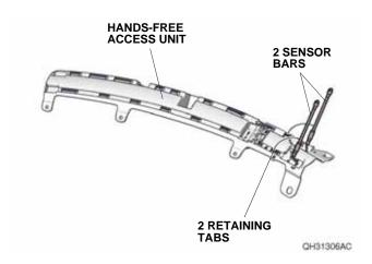
46. While wearing eye protection, use an air saw to cut the hands-free access unit along the scribe line. Remove any burrs.
