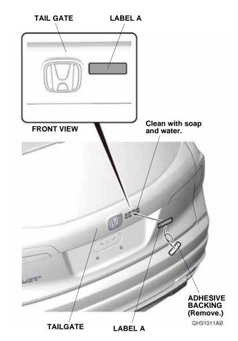
60. Remove the adhesive backing from the label A, and attach the label A to the tailgate as shown.
