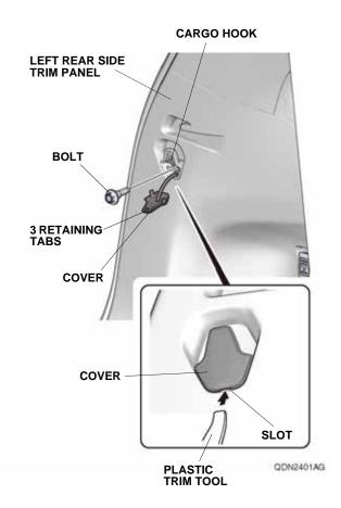
13. Using a plastic trim tool, pull the cover, and remove the screw.
