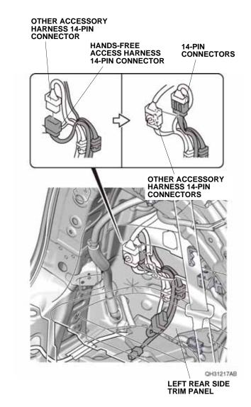
32. Secure the 14-pin connectors to the other accessory harness 14-pin connectors as shown.
