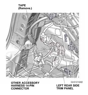
31. Plug the other accessory harness 14-pin connector into the hands-free access harness 14-pin connector.
