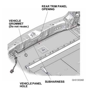
38. Secure the grommet on the subharness to the vehicle panel hole.
