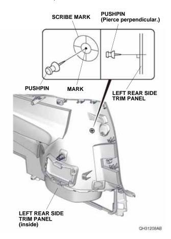
20. While wearing eye protection, drill the pierced mark on the left rear side trim panel using a 3 mm drill bit. Enlarge the 3 mm hole to 26 mm using a 26 mm hole saw, and remove any burrs.
