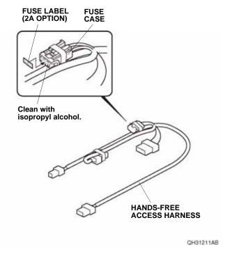
Plug the hands-free access harness 3-pin connector into the switch.
