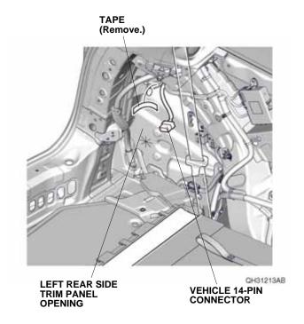
28. Route the hands-free access harness as shown, and plug the vehicle 14-pin connector into the hands-free access harness 14-pin connector.
