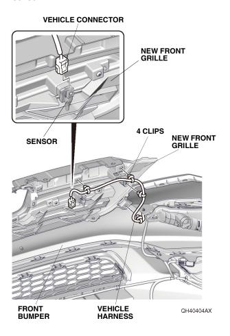
15. Install the front bumper. Install the new front upper grille to the front bumper with 10 clips, four retaining tabs, and four bolts.
