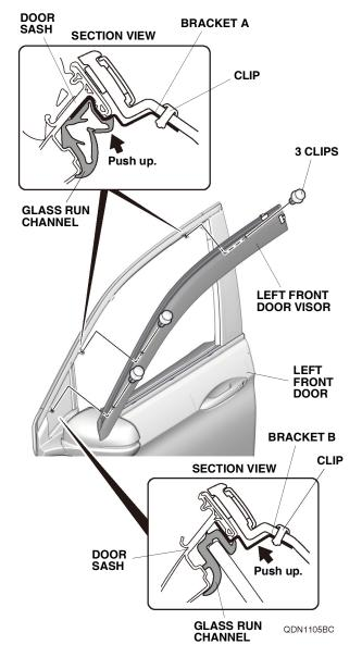
8. Using the three clips, secure the left front door visor to the two brackets A and one bracket B as shown.
