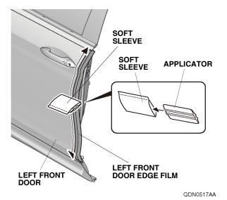
Slowly remove the protective film from the left front door edge film.
