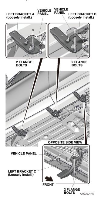
4. With the help of an assistant, install the left running board to the left bracket A, left bracket B, and left bracket C with six flange bolts. Torque the flange bolts to 20 lb-ft (27 N·m).
