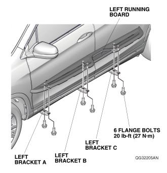
5. Tighten the six flange bolts loosely installed in step3. Torque the flange bolts to 20 lb-ft (27 N·m).
