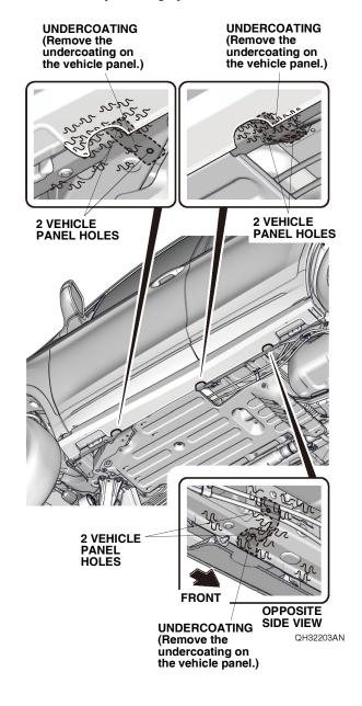
Loosely install the left bracket A, left bracket B, and left bracket C to the vehicle panel with six flange bolts
