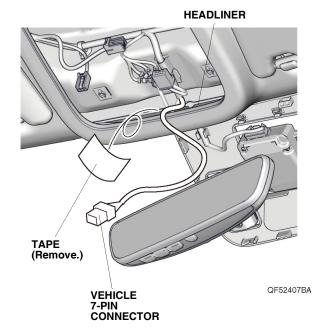
8. Attach masking tape to the vehicle harness at the measurement shown.
