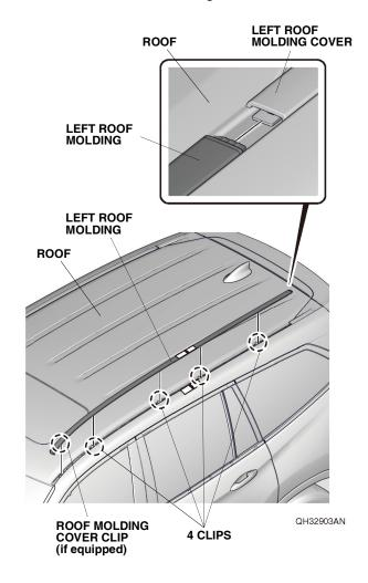
5. Remove the four molding clips from either the left roof molding or the roof stud bolts.
