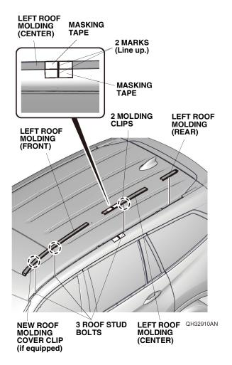
12. Install the nut to the roof stud bolt. Torque the nut to 7 lb-ft (10 N·m).
