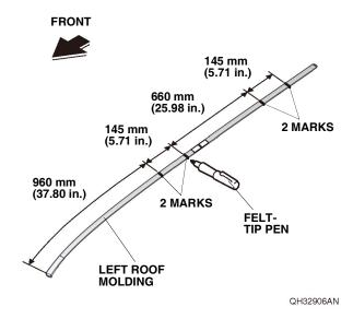
8. While wearing eye protection, use an air saw to cut the left roof molding at the four marks. Remove any burrs.
