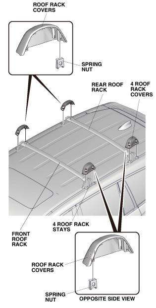
19. Secure each roof rack cover to the four roof rack stays with one self-tapping screw as shown.
