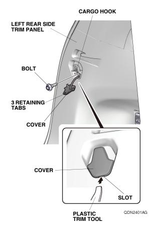
Using a plastic trim tool, pull the cover and remove the screw.
