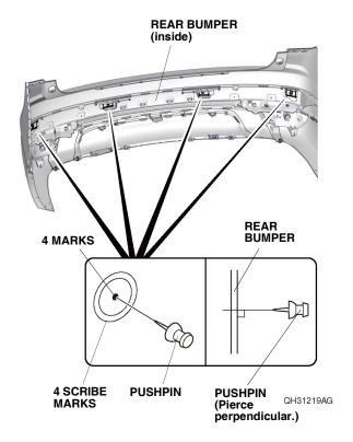
59. While wearing eye protection, drill the four pierced marks to 8.5 mm from the inside of the rear bumper. First, drill with a 3 mm drill bit, then follow with a 6 mm drill bit, and finish with an 8.5 mm drill bit. NOTE: Make sure to drill perpendicular to the rear bumper.
