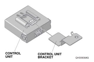
Install the control unit to the vehicle panel with one flange bolt as shown.
