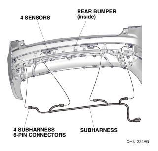
65. Secure the subharness to the rear bumper with four wire ties with clip A and four holders as shown.
