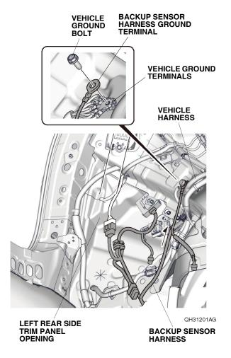
31. Secure the backup sensor harness to the vehicle harness with three wire ties.
