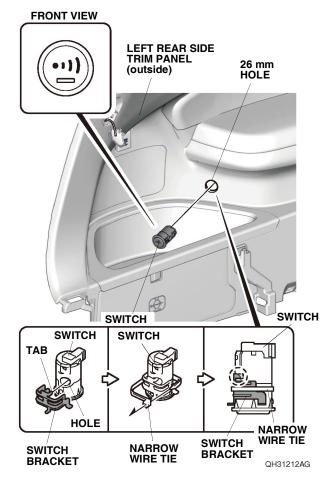
48. Line up the tab on the switch bracket with the hole on the switch and secure the switch bracket to the switch with one narrow wire tie.
