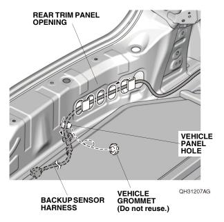
39. Secure the grommet on the backup sensor harness to the vehicle panel hole.
