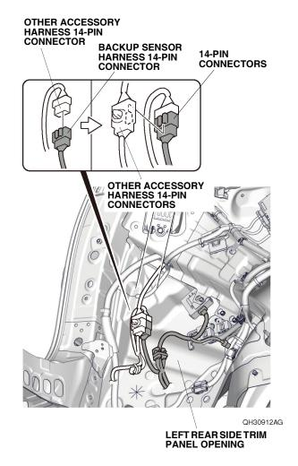
29. Install the 14-pin connectors to the other accessory harness 14-pin connectors as shown.
