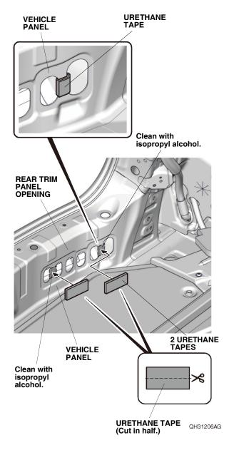
37. Using scissors, cut one urethane tape in half, and attach the two pieces to the vehicle panel as shown.
