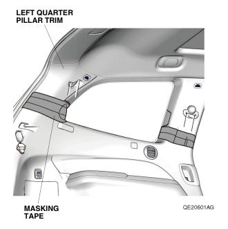
15. Remove the left rear side trim panel, and unplug the vehicle connector (if equipped).
