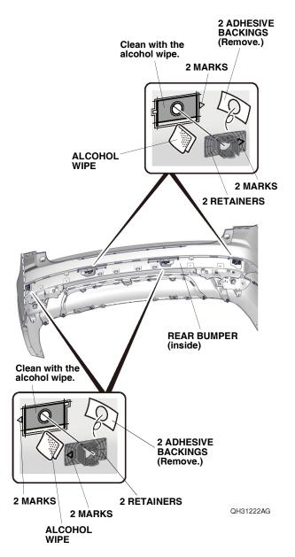
62. Remove the four adhesive backings from the four retainers, and attach the four retainers to the rear bumper as shown.
