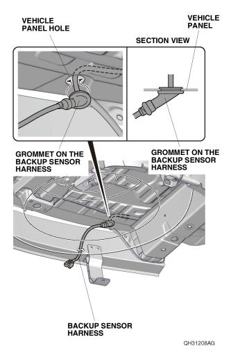
40. Secure the backup sensor harness to the vehicle panel with two wire ties as shown.
