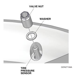
2. Remove and discard the grommet from the tire pressure sensor.
