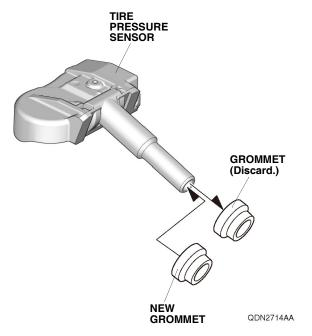
3. Install the new grommet onto the tire pressure sensor.
