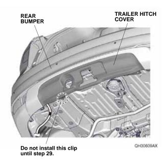
27. With the help of an assistant, bring the trailer hitch close to the vehicle, install the socket harness 7-pin socket to the trailer hitch with one 6 x 16 mm flange bolt, one 6 x 19 mm shoulder bolt, and two flange nuts.
