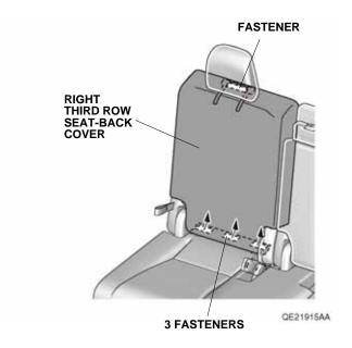
5. Secure the right third row seat-back cover with the fastener. Secure the strap to the right third row seat-back cover with the fastener.
