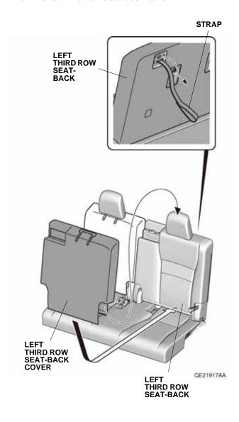
7. Secure the left third row seat-back cover with the fasteners.
