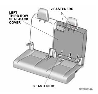
8. Secure the left third row seat-back cover with the fastener. Secure the strap to the left third row seat-back cover with the fastener.
