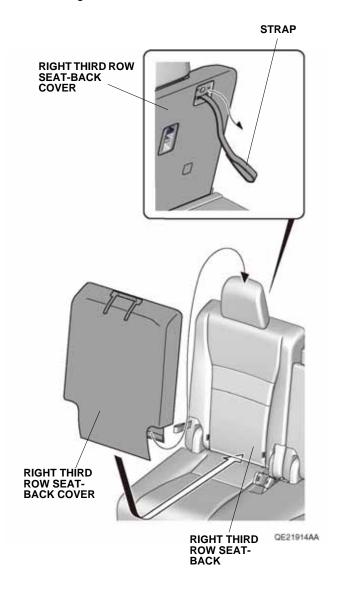
4. Secure the right third row seat-back cover with the fasteners.
