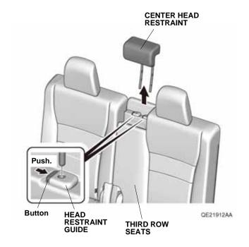
2. Install the center head restraint cover.
