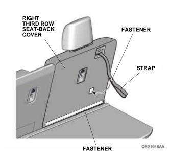
6. Install the left third row seat-back cover to the left third row seat-back. Pull the strap through the hole on the left third row seat-back cover.
