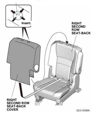
4. Secure the right second row seat-back cover with the fasteners.
