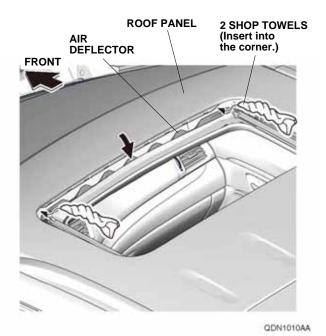
Open the moonroof. Roll up two shop towels, and insert them between the roof panel and air deflector to lower the air deflector. Be careful not to damage the air deflector. 3. Measure and make two marks on the roof panel at the measurements shown.
