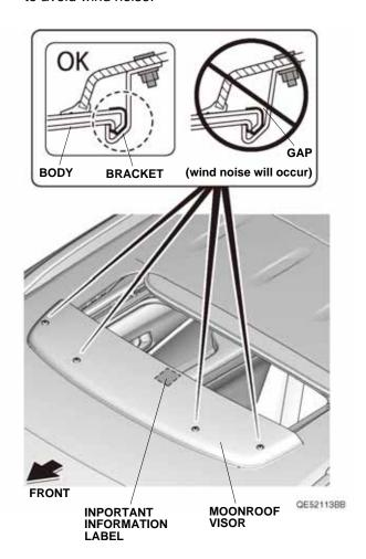
13. Position the moonroof visor with equal spacing on each side. Check that the rubber molding is not twisted or rolled under the moonroof visor.
