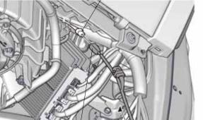
RIGHT RUNNING BOARD HARNESS 2-PIN CONNECTOR 40. Secure the right running board harness to the vehicle harness with two wire ties.
