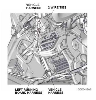
29. Secure the left running board harness to the vehicle harness with two wire ties.
