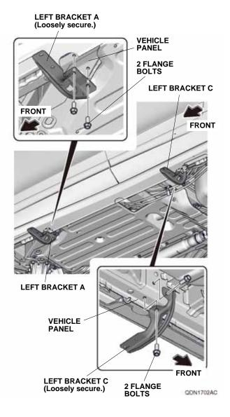
12. Secure the left running board to the left bracket A and left bracket C with four flange bolts. Torque the flange bolts to 27 N·m (20 lb·ft).
