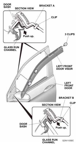
Using the three clips, secure the left front door visor to the two brackets A and one bracket B as shown. Make sure to push up on the two brackets A and one bracket B while installing three clips. NOTE: Be extremely careful when installing the clips; they cannot be reinstalled after installation. 9. Open the left front door. Line up the left front door visor as shown.
