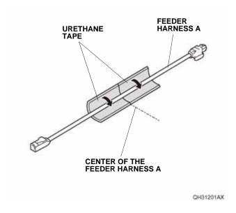
22. Route the feeder harness A as shown. Plug the feeder harness A connector into the vehicle feeder connector.
