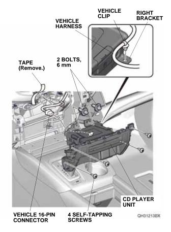
35. Install the CD player unit to the dashboard with the four self-tapping screws removed in step 18 and two 6 mm bolts.
