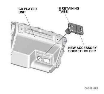
30. Install the accessory socket to the new accessory socket holder with two retaining tabs.
