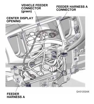
23. Secure the feeder connectors and CD player harness to the vehicle harness with one wire tie.
