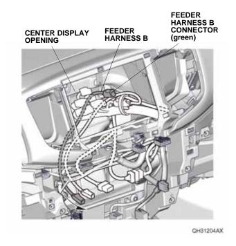
Plug the feeder harness B connector into the infotainment control unit. Install the center display.
