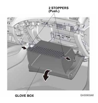
7. Remove the glove box, and unplug the vehicle connector.
