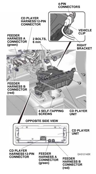
33. Install the CD player unit to the dashboard with the four self-tapping screws removed in step 18 and two 6 mm bolts. Go to step 36.
