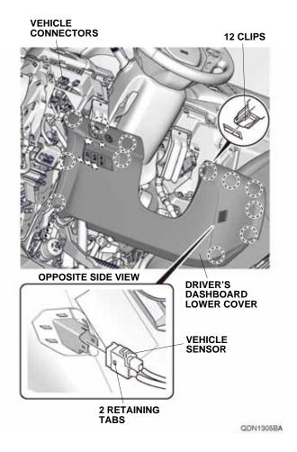
Remove the center upper panel, and unplug the vehicle connector.
