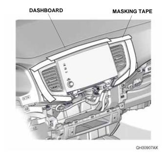
13. Loosen the two bolts. Remove the center display, and unplug the vehicle connectors.
