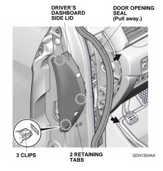
9. Remove the driver's dashboard lower cover, and unplug the vehicle connectors, and release the vehicle sensor.
