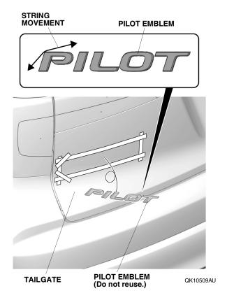
10. Install the PILOT emblem in the guide form, and temporarily secure it with masking tape.
