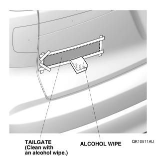
12. Remove the adhesive backing from the PILOT emblem. Line up the guide form with the masking tape, and attach the PILOT emblem to the tailgate.
