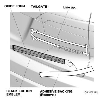
Remove the guide form and using the palm of your hand, firmly press the BLACK EDITION emblem against the tailgate for 30 seconds.
