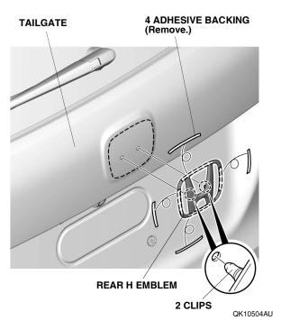
4. Using the palm of your hand, firmly press the rear H emblem against the tailgate for 30 seconds.
