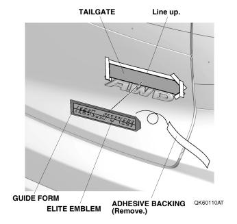
39. Remove the guide form and using the palm of your hand, firmly press the ELITE emblem against the tailgate for 30 seconds.
