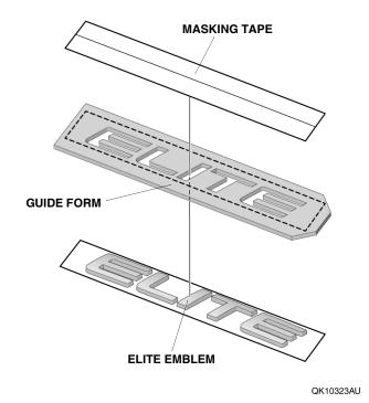
37. Using an alcohol wipe, thoroughly clean the tailgate where the ELITE emblem will attach.
