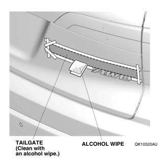
28. Remove the adhesive backing from the BLACK EDITION emblem. Line up the guide form with the masking tape, and attach the BLACK EDITION emblem to the tailgate.
