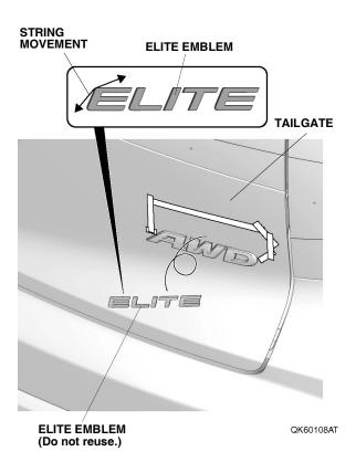
36. Install the ELITE emblem in the guide form, and temporarily secure it with masking tape.
