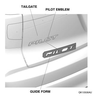
7. Attach masking tape along the guide form as shown.
