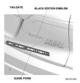
23. Attach masking tape along the guide form as shown.
