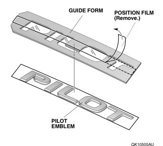
6. Install the guide form to the PILOT emblem on the tailgate.
