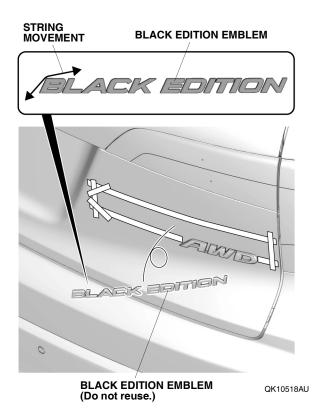
26. Install the BLACK EDITION emblem in the guide form, and temporarily secure it with masking tape.
