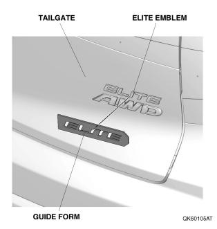
33. Attach masking tape along the guide form as shown.
