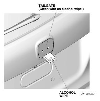
3. Remove the adhesive backings from the rear H emblem. Install the rear H emblem to the tailgate as shown.
