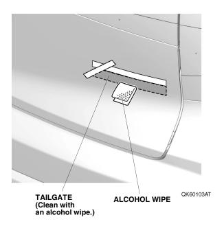
18. Remove the adhesive backing from the AWD emblem. Line up the AWD emblem with the masking tape, and attach the AWD emblem to the tailgate.
