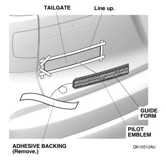
13. Remove the guide form and using the palm of your hand, firmly press the PILOT emblem against the tailgate for 30 seconds.
