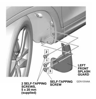
5. While holding the left front splash guard against the left front inner fender, tighten self-tapping screws in the order shown.
