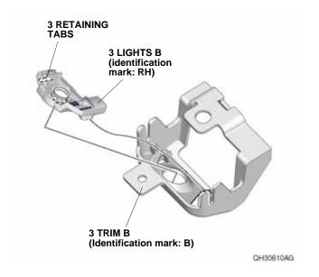
17. Install the three retainers to each trim B with three self-tapping screws as shown.
