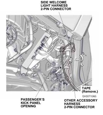
50. Bundle up the excess side welcome light harness, and secure it and 2-pin connectors to the vehicle harness with two wire ties as shown.
