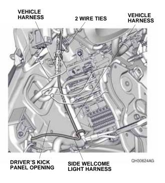
32. Secure the side welcome light harness to the vehicle harness with two wire ties. Go to step 35.
