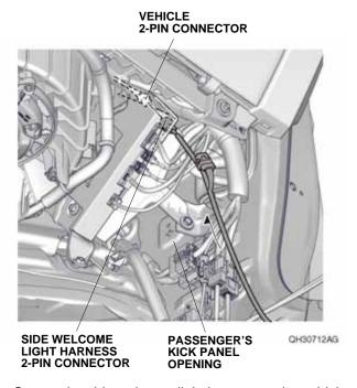
47. Secure the side welcome light harness to the vehicle harness with two wire ties.
