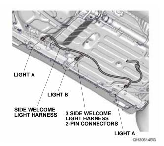
21. Secure the side welcome light harness to the two trim A, one trim B, and left side sill panel with seven wire ties as shown.
