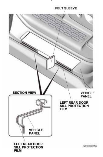
21. Using a shop towel, wipe off the 3M protective tape application solution. Allow the left rear door sill protection film to dry thoroughly. Remove the masking tape.
