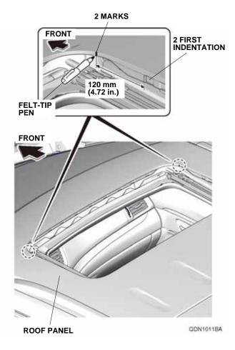
Using isopropyl alcohol on a shop towel, clean the roof panel at each of the two marks you have made but do not wipe off the marks.
