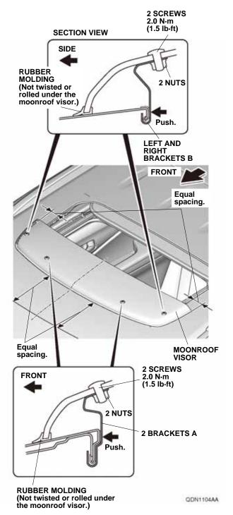
14. Tighten the two screws and two nuts on the front of the vehicle first, then tighten the two screws and two nuts on each side. Tighten while applying pressure so that there is no gap between the roof panel and the brackets A and B. Torque the screws to 2.0 N·m (1.5 lb·ft).  Remove the shop towels inserted in step 2. Remove the IMPORTANT INFORMATION label.
