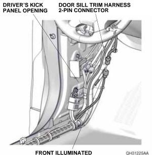
FRONT ILLUMINATED DOOR SILL TRIM HARNESS 2-PIN CONNECTOR 56. Bundle up the excess front illuminated door sill trim harness, and secure it and the 2-pin connectors to the vehicle harness with three wire ties as shown.
