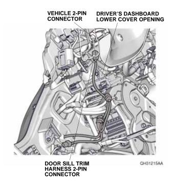
43. Secure the door sill trim harness to the vehicle harness with two wire ties.
