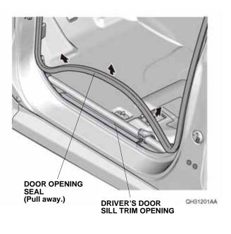
20. Using an alcohol wipe, thoroughly clean the vehicle panel where the front illuminated door sill trim will attach.
