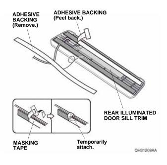
30. Line up the rear illuminated door sill trim with the masking tape. Attach the rear illuminated door sill trim to the vehicle panel.
