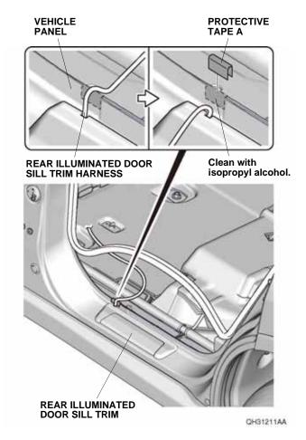
35. Install the protective clip to the protective tape A on the vehicle panel.
