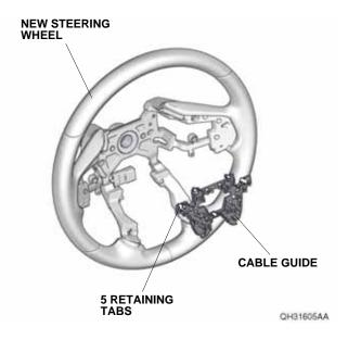
30. Install the new cable reel cord to the cable guide with one washer-screw removed in step 27. Plug the new cable reel cord 4-pin connector into the new steering wheel 4-pin connector, and secure the new cable reel cord to the cable guide.
