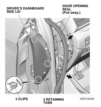
4. Remove the driver's dashboard lower cover, and unplug the vehicle connectors, and release the vehicle sensor.
