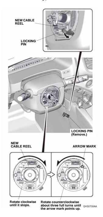
37. Before installing the new steering wheel, make sure the front wheels are still pointing straight-ahead. To confirm the cable reel is line up properly, rotate the cable reel clockwise until it stops, then rotate it counterclockwise about three full turns. The arrow mark on the new cable reel label must point straight up.
