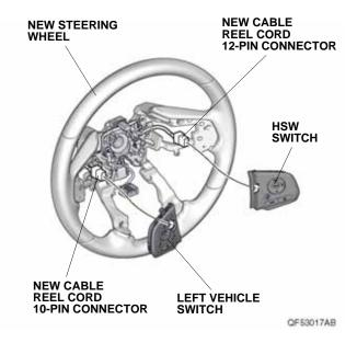
Install the control unit on the center spoke trim with two 4 x 14 mm TORX screws.
