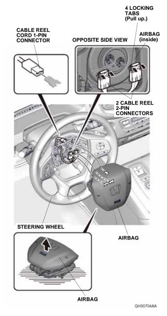
7. Remove the airbag. Do not drop the removed airbag or hit it on an object. Place the removed airbag in a safe place with the padded surface (top) facing up.
