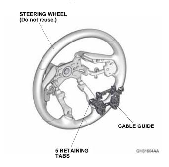
29. Install the cable guide on the new steering wheel with five retaining tabs.
