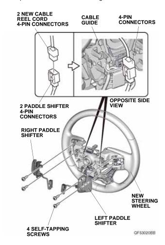
35. Install the steering wheel cover on the new steering wheel with four self-tapping screws removed in step 23 and two retaining tabs.
