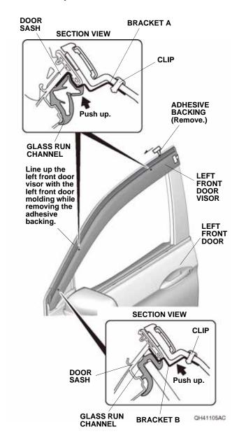
12. Using a rubber roller, apply firm pressure against the left front door visor and roll from one end to the other. NOTE: Apply firm pressure, especially at the ends.
