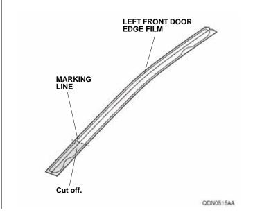
Open the left front door again. Peel back about 50 mm (1.97 in.) of adhesive backing from the left front door edge film. Line up the V-notch in the left front door edge film with the character line of the left front door.
