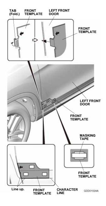
2. Line up the middle template with the character line, and attach it to the left front door and left rear door with strips of masking tape as shown.
