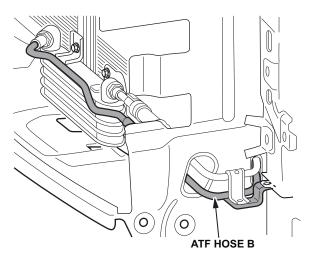
14. Install the hose bracket using a 6 x 16 mm washer bolt.
