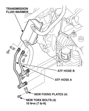
Make sure the connection points are clean and free of debris, then install ATF pipe A and ATF pipe B using the new fixing plates and Torx bolts supplied in this kit.
