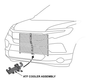
9. Install the ATF cooler with three 6 x 20 mm washer bolts.
