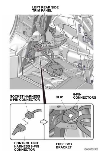
36. Secure the 8-pin connectors to the fuse box bracket with the clip on the control unit harness 8-pin connector.
