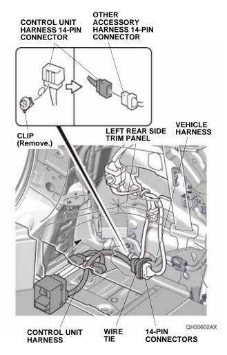
18. Secure the 14-pin connectors to the vehicle harness with one wire tie.
