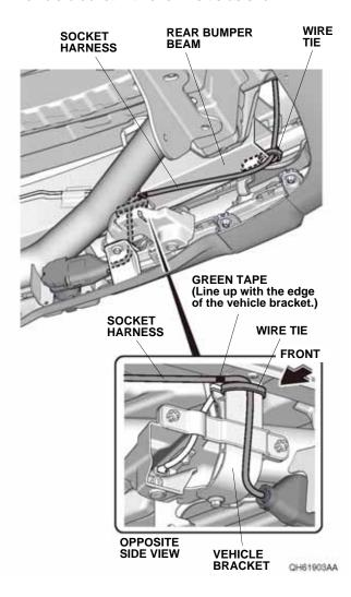
31. Secure the socket harness to the rear bumper beam with one wire tie. Go to step 34.
