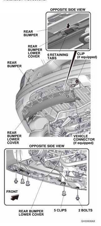
23. Remove the rear bumper lower cover, and unplug the vehicle connector (if equipped).
