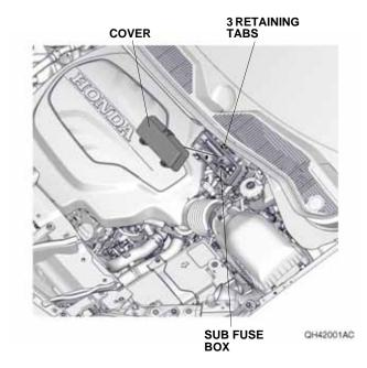
43. Plug the two 20A blade fuses and the 30A block fuse into the sub fuse box.
