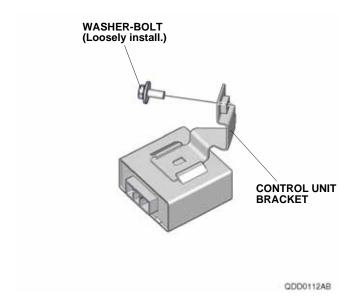
9. Install the control unit to the vehicle panel as shown.
