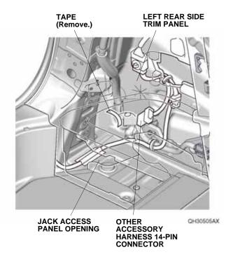
14. Remove the clip from the control unit harness 14-pin connector. Route the control unit harness 14-pin connector, and plug the other accessory harness 14-pin connector into the control unit harness 14-pin connector.
