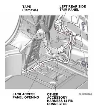
Remove the clip from the control unit harness 14-pin connector. Route the control unit harness 14-pin connector, and plug the other accessory harness 14pin connector into the control unit harness 14-pin connector.
