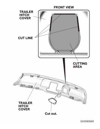
Install the trailer hitch cover as described in the trailer hitch installation instructions.
