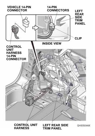
12. Secure the 14-pin connectors to the back of the left rear side trim panel with the clip on the control unit harness 14-pin connector. Go to step 20.
