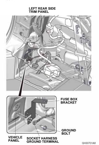
35. Plug the socket harness 8-pin connector to the control unit harness 8-pin connector.
