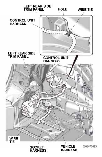
Secure the socket harness to the vehicle harness with one wire tie.
