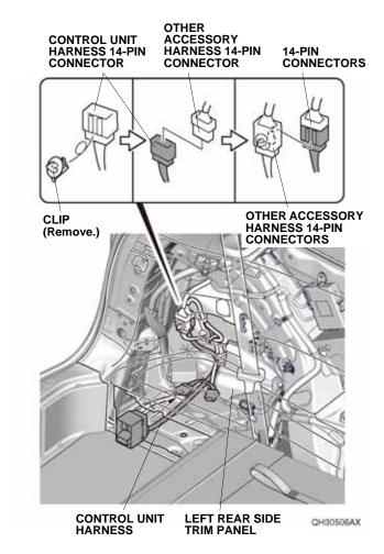
15. Secure the 14-pin connectors to the back of the other accessory harness 14-pin connectors. Go to step 20.
