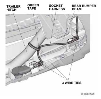
33. Secure the socket harness to the rear bumper beam with two wire ties.
