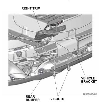
37. Install the right bracket to the right trim with two clips removed in step 9.
