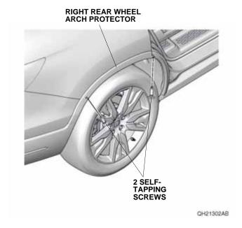
11. Remove the two self-tapping screws.
