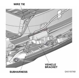
46. Secure the subharness, rear welcome light harness, and 2-pin connectors to the vehicle bracket with one wire tie as shown. Go to step 60.
