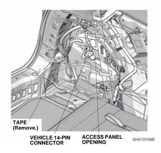
17. Route the rear welcome light harness, and plug the vehicle 14-pin connector into the rear welcome light harness 14-pin connector.
