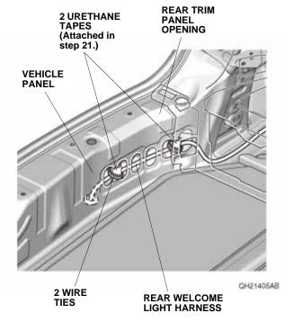
25. Using isopropyl alcohol on a shop towel, thoroughly clean the vehicle panel where the aluminum tape will attach.
