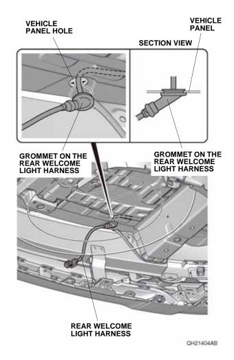
24. Secure the rear welcome light harness to the vehicle panel with two wire ties as shown.
