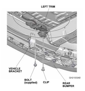
41. Install the left bracket to the left trim with two clips A (long).
