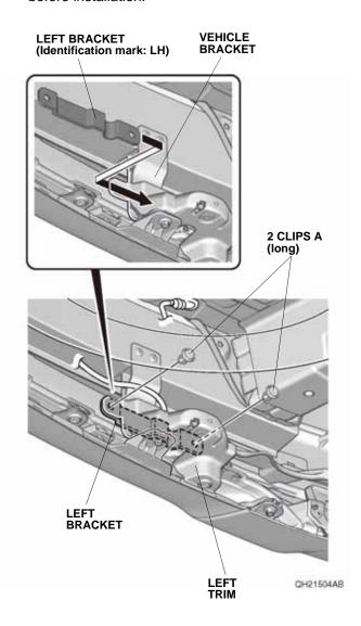
42. Route the subharness. Plug the rear welcome light harness 2-pin connector into the subharness 2-pin connector.
