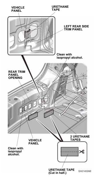
21. Using scissors, cut one urethane tape in half, and attach them to the vehicle panel as shown.
