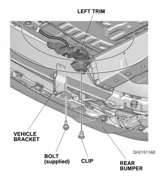
56. Install the left bracket to the left trim with two clips A (long).
