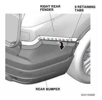
• With the help of an assistant, release the two retaining tabs on each side.
