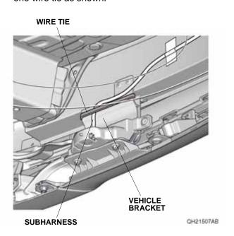
60. Secure the subharness to the vehicle bracket with one wire tie as shown.
