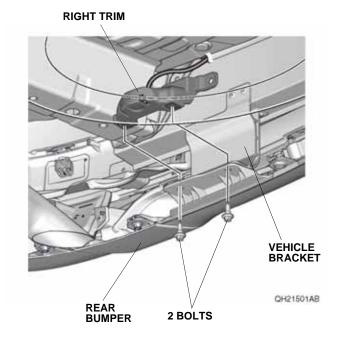
52. Install the right bracket to the right trim with the two clips removed in step 14.
