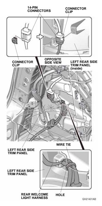
19. Secure the rear welcome light harness to the left rear side trim panel with one wire tie as shown.
