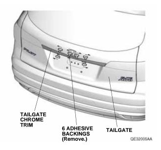
Using a rubber roller, apply firm pressure against the tailgate chrome trim and roll from one end to the other. Apply firm pressure especially at the ends.
