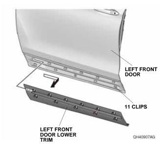
3. Remove the eleven clips from the door as shown.
