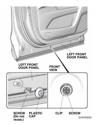
2. Slide the left front door lower trim back and out to remove it.
