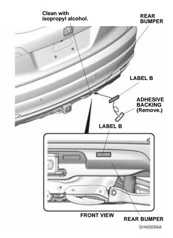
62. Remove the adhesive backing from the label B, and attach the label B to the rear bumper as shown. NOTE: Make sure the customer is aware that label B can be removed after reading.
