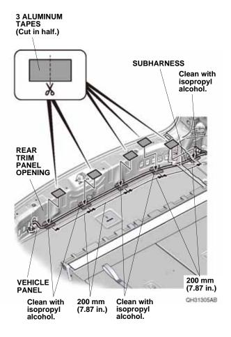
42. Using scissors, cut three aluminum tapes in half, and secure the subharness to the vehicle panel with five pieces of aluminum tape as shown.
