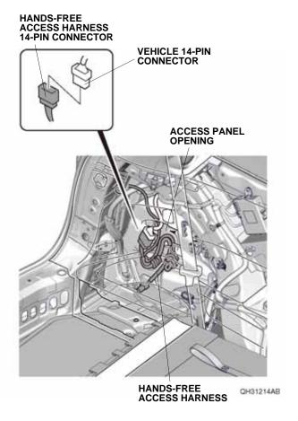
29. Install the connector clip to the 14-pin connectors. Secure the 14-pin connectors to the left rear side trim panel with the connector clip on the 14-pin connectors. Go to step 33.
