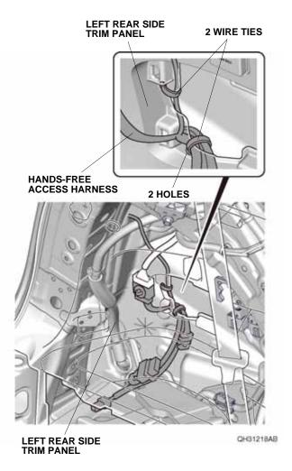
34. Route the subharness as shown. Plug the handsfree access harness 2-pin connector into the subharness 2-pin connector.
