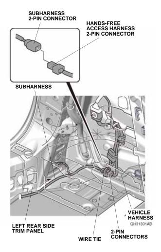
35. Secure the 2-pin connectors to the vehicle harness with one wire tie.
