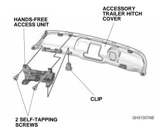
52. Plug the subharness 3-pin connector into the handsfree access unit. Install the rear bumper lower cover or accessory trailer hitch cover.
