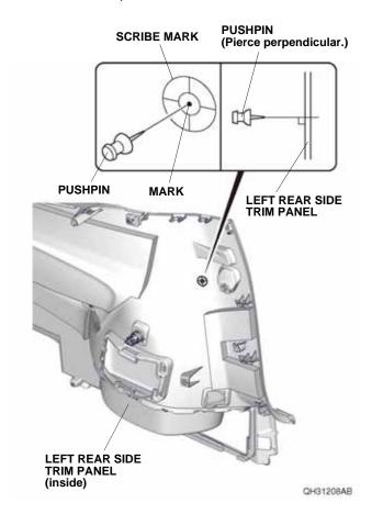
20. While wearing eye protection, drill the pierced mark on the left rear side trim panel using a 3 mm drill bit. Enlarge the 3 mm hole to 26 mm using a 26 mm hole saw, and remove any burrs.
