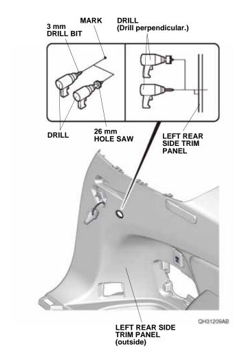
21. Install the switch into the 26 mm hole.
