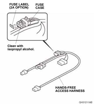
24. Plug the hands-free access harness 3-pin connector into the switch.
