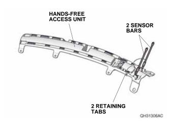
46. While wearing eye protection, use an air saw to cut the hands-free access unit along the scribe line. Remove any burrs.
